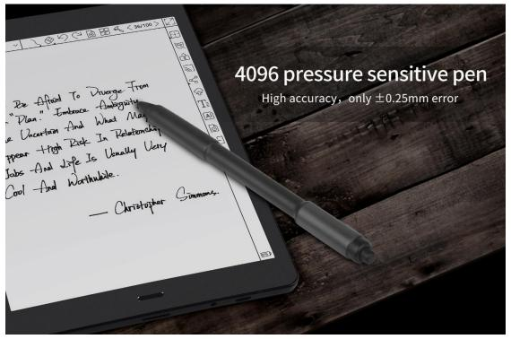
Use Wacom electromagnetic stylus, support 4096 level pressure sense, no need to charge, pen smart and smooth, can reproduce the handwriting track. The writing effect is almost the same as the paper.
